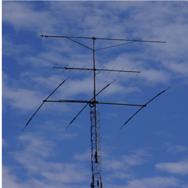
Figure 20.3: A Yagi–Uda beam antenna: driven element, reflector, and directors.
